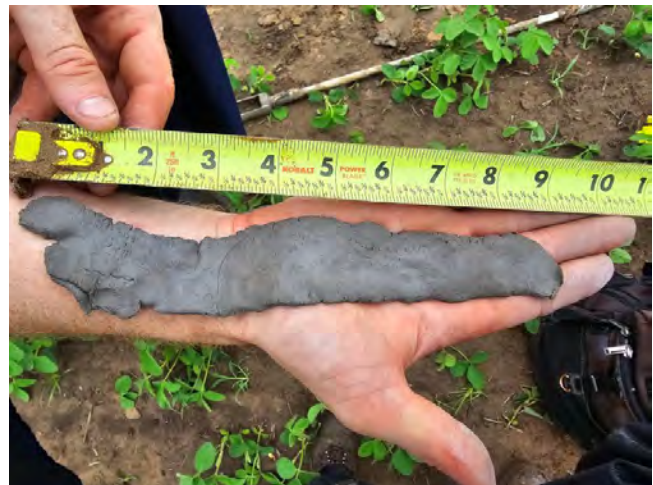
W-8 (showing clay that is present 35-inches below the surface)
