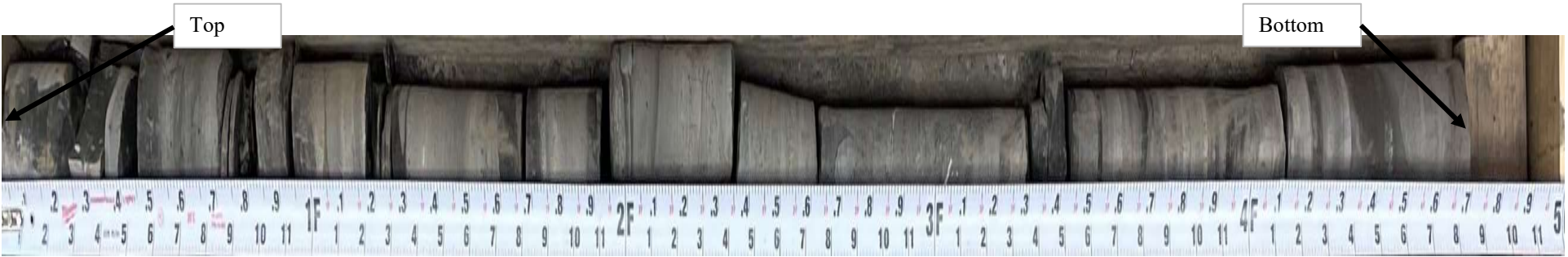
Photograph 151 Boring B-630 Run 1 Depth 22.0' - 27.0' See Photographs Nos. 152 and 153 for detailed views.
