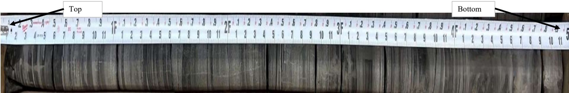
Photograph 100 Boring: B-588 Run 2 Depth 16.0'- 21.0' See Photographs Nos. 101 and 102 for detailed views.
