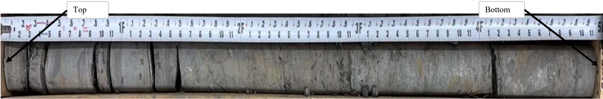
Photograph 166 Boring B-664 Run 2 Depth 30.1' - 35.1' See Photographs Nos. 167 and 168 for detailed views.
