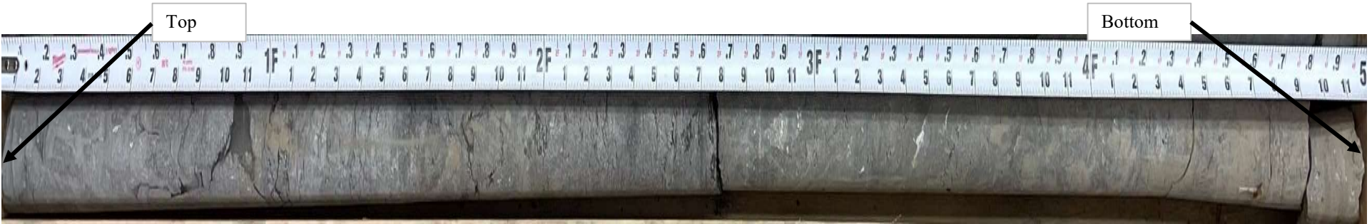
Photograph 76 Boring B-561 Run 2 Depth 25.4' -30.4' See Photographs Nos. 77 and 78 for detailed views.
