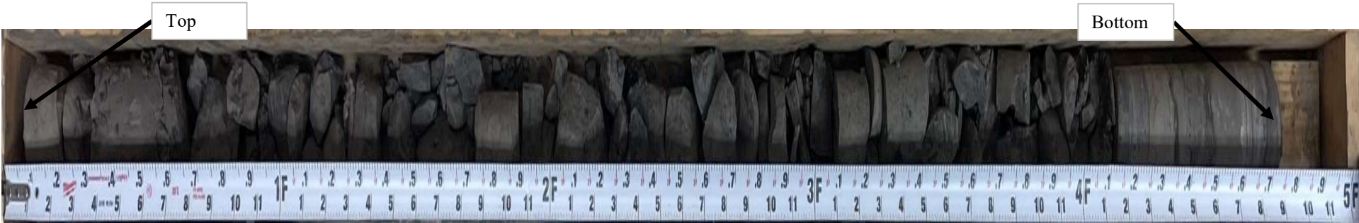
Photograph 127 Boring: B-612 Run 1 Depth 23.6' - 28.6' See Photographs Nos. 128 and 129 for detailed views.
