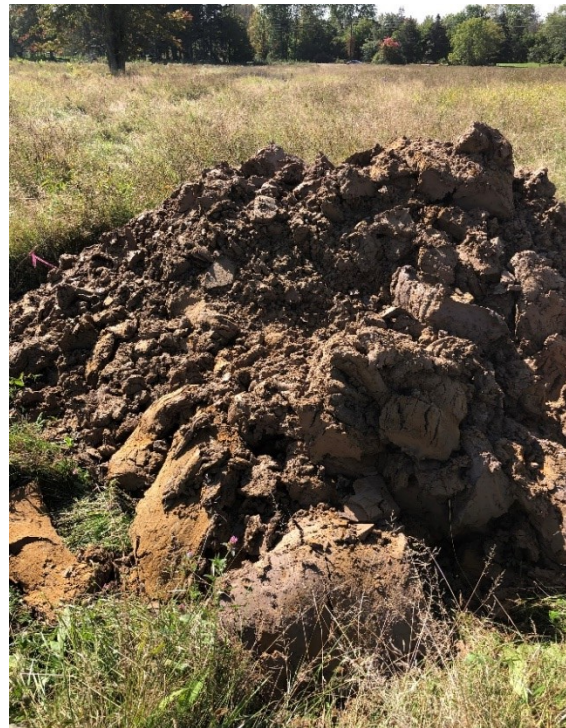
Figure 12: Materials Excavated from Test Pit TP-6
