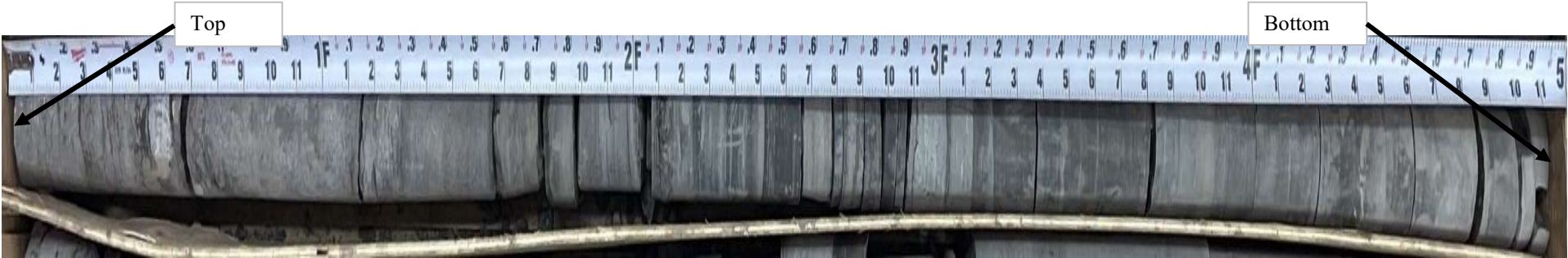
Photograph 82 Boring B-565 Run 2 Depth 23.0' - 28.0' See Photographs Nos. 83 and 84 for detailed views.
