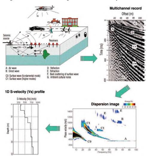
Figure 1. Overall procedure for data collection and processing.
