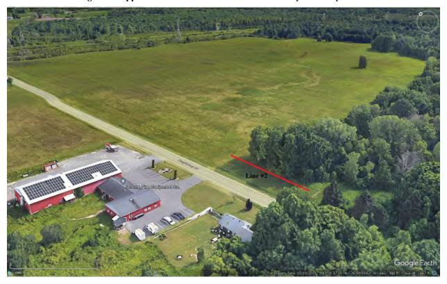
Figure 8. Approximate Location of Surface-wave Analysis Survey Line 2
