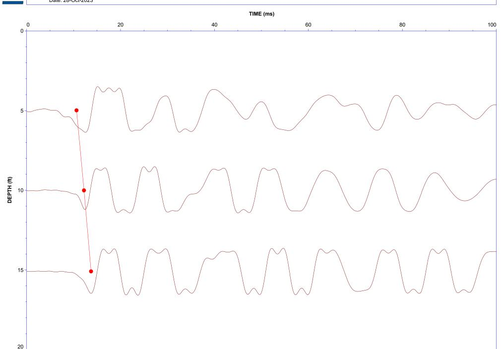
Seismic Cone Penetration Test Compression Wave (Vp)
