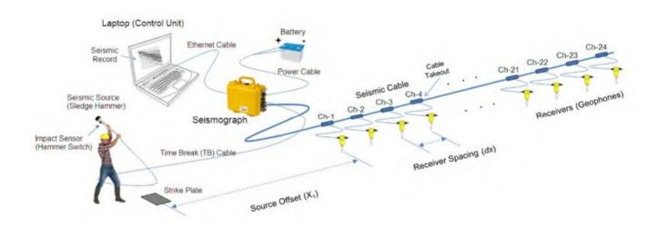
Figure 2. Typical field configuration with an active source survey.
