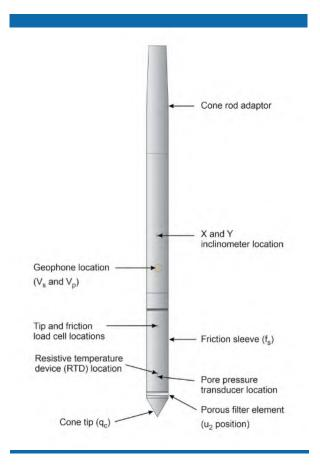
Figure CPTu. Piezocone Penetrometer (15 cm²)
