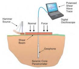
Figure SCPTu-1. Illustration of the SCPTu system
