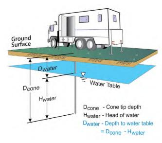
Figure PPD-1. Pore pressure dissipation test setup
