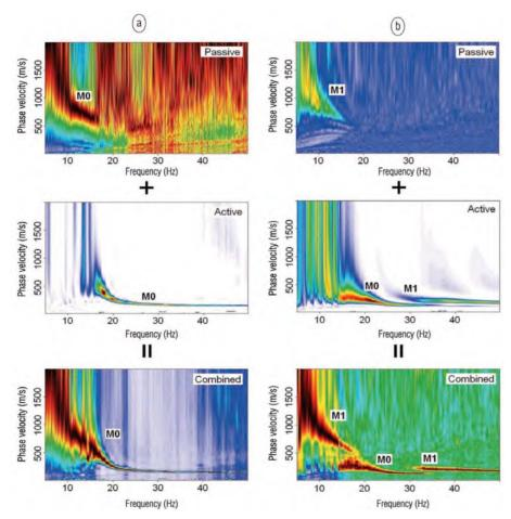
Figure 3. Dispersion images from passive and active sources are combined to enlarge dispersion bandwidth.
