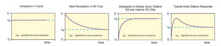
Figure PPD-2. Pore pressure dissipation curve examples
