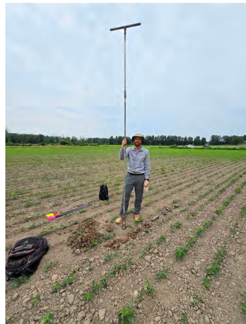
Reed 1 (digging a deep test hole using a 10.5-foot-long soil auger)
